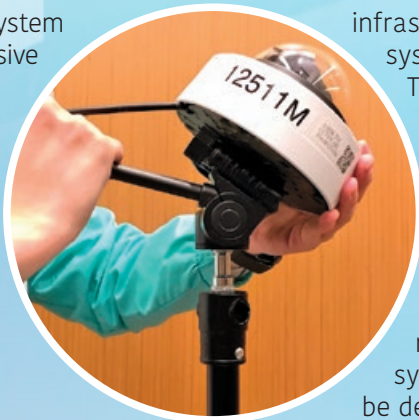
The surveillance camera is mounted onto a free-standing pole for fast and flexible deployment. 監察攝影機安裝在獨立支架上，可快捷靈活地調動。
