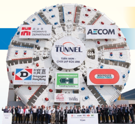
A 17.6m diameter TBM, the world's largest at the time of construction, is deployed for the road tunnel section of the three-lane configuration. 工程採用了全球最大、直徑17.6米的隧道鑽挖機，以建造可供三線行車的隧道路段。
