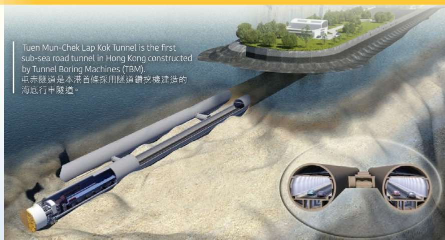
A 17.6m diameter TBM, the world's largest at the time of construction, is deployed for the road tunnel section of the three-lane configuration. 工程採用了全球最大、直徑17.6米的隧道鑽挖機，以建造可供三線行車的隧道路段。
