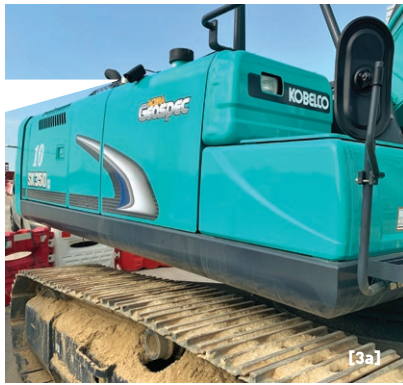
【3a】 I-Vision Smart Monitoring System excavators are equipped with a 360-degree CCTV view with cameras to enhance its operational safety. [I-Vision] 智能監控系統挖掘機配備360度閉路電視監察，提升操作安全。
