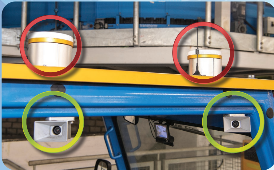
Differential Global Positioning System (red circle) and high-definition cameras (green circle) are equipped on the AET featuring improved location accuracy rate.
